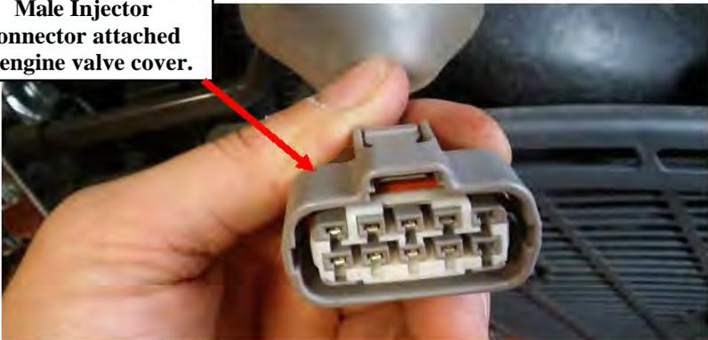
**3)** On the Ag Diesel Solutions module harness, the white 10 pin male injector connector will connect to the female injector connector fixed on the valve cover as seen in Step 1. The module harness can be routed along existing wire loom.
