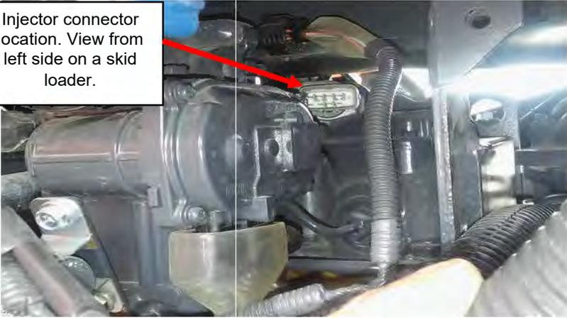
2) Unplug the stock injector connector. Press and hold the release tab on the connector and gently pull the connector apart.
