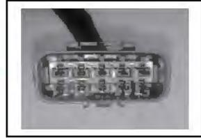
**5)** Locate the stock EGR valve connector and disconnect. Depending on the engine orientation, this will be accessible from one point in the engine compartment (as shown from the left). This is a four pin connector.
