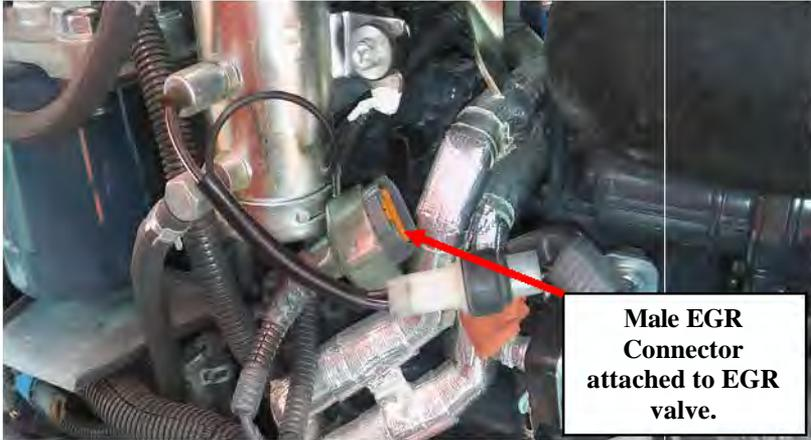
**7) Plug the male EGR Valve connector from the module harness into the EGR Valve. Plug the stock male EGR Valve connector into the Ag Diesel Solutions female EGR Valve connector of the harness.**
